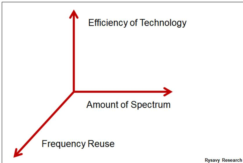
The progression of wireless technology has addressed each of these variables, harnessing ever more spectrum, improving efficiency in each new generation, and increasing the number of cells. A number of technology and market developments are enabling these advances:
