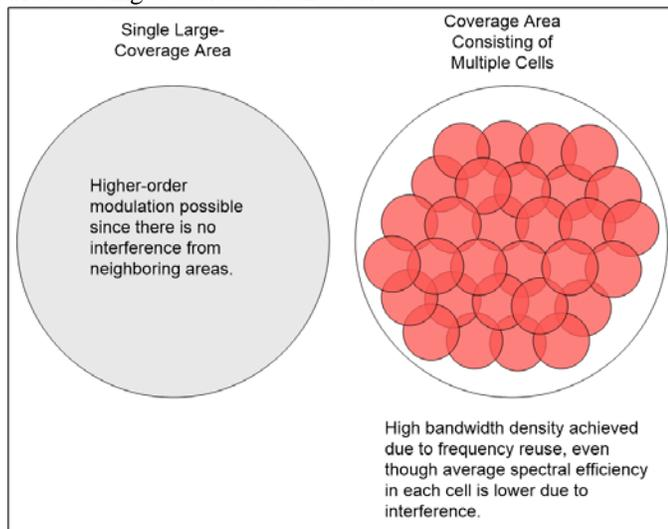
**Figure 3: Comparison of TV Broadcasting and Cellular Use of Spectrum.**
