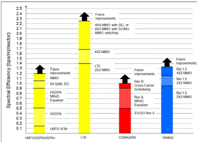
**Figure 2: Comparison of Downlink Spectral Efficiency.**
