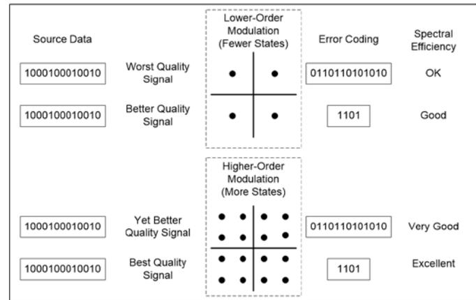
**Figure 1. Example of Dynamic Modulation and Coding.**
