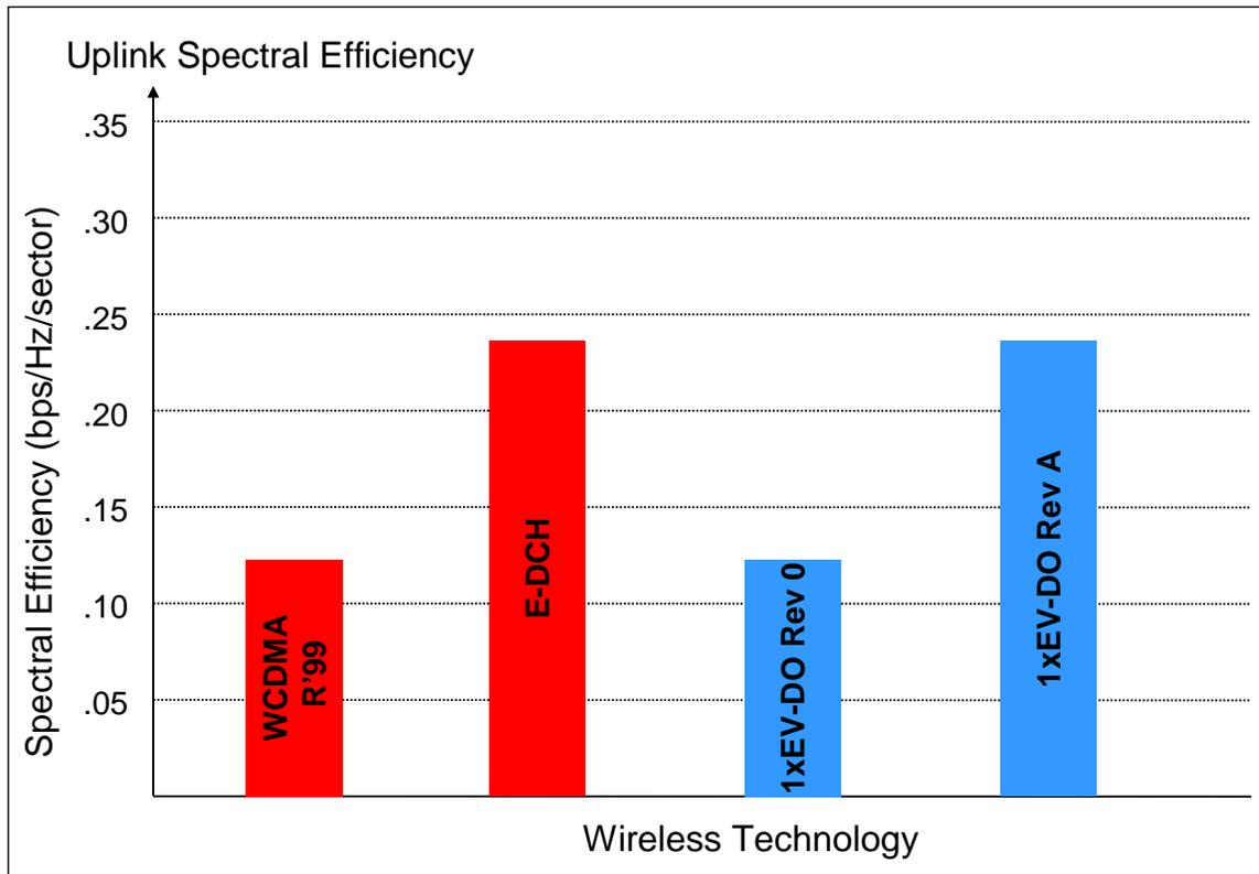
The Enhanced Dedicated Channel for UMTS significantly increases uplink capacity, as does Rev A for 1xEV-DO compared to Rev 0. OFDM-based systems exhibit slightly improved uplink capacity relative to CDMA technologies.
