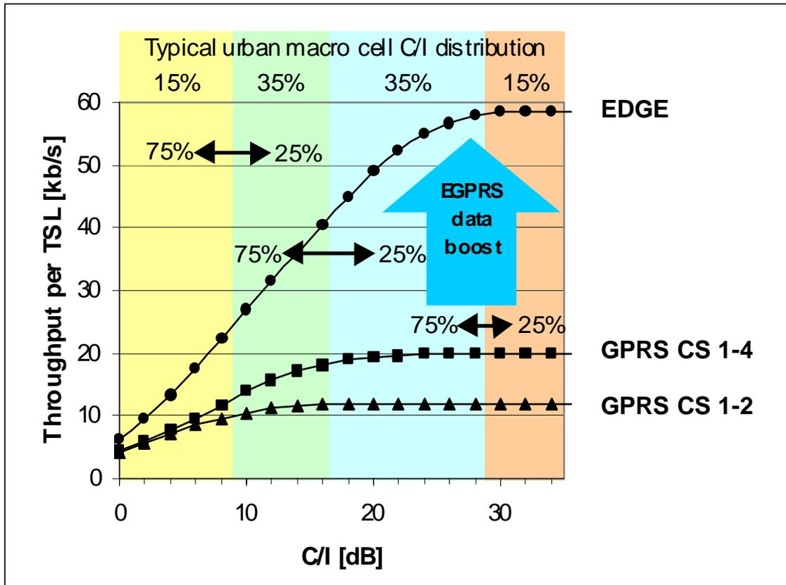
In Figure 5, the horizontal double-tipped arrows show how the 15%, 50% and 85% colored borders that depict the C/I distribution in the cell shift depending on network load<sup>31</sup>. The diagram uses a 50% network load, and the arrows show how C/I and throughputs vary between 25% and 75% network load.
