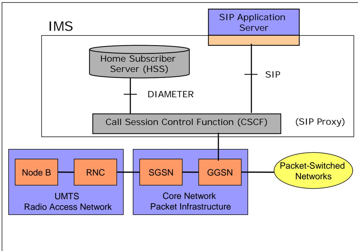
The benefits of using IMS include handling all communication in the packet domain, tighter integration with the Internet, and a lower cost infrastructure that is based on IP
