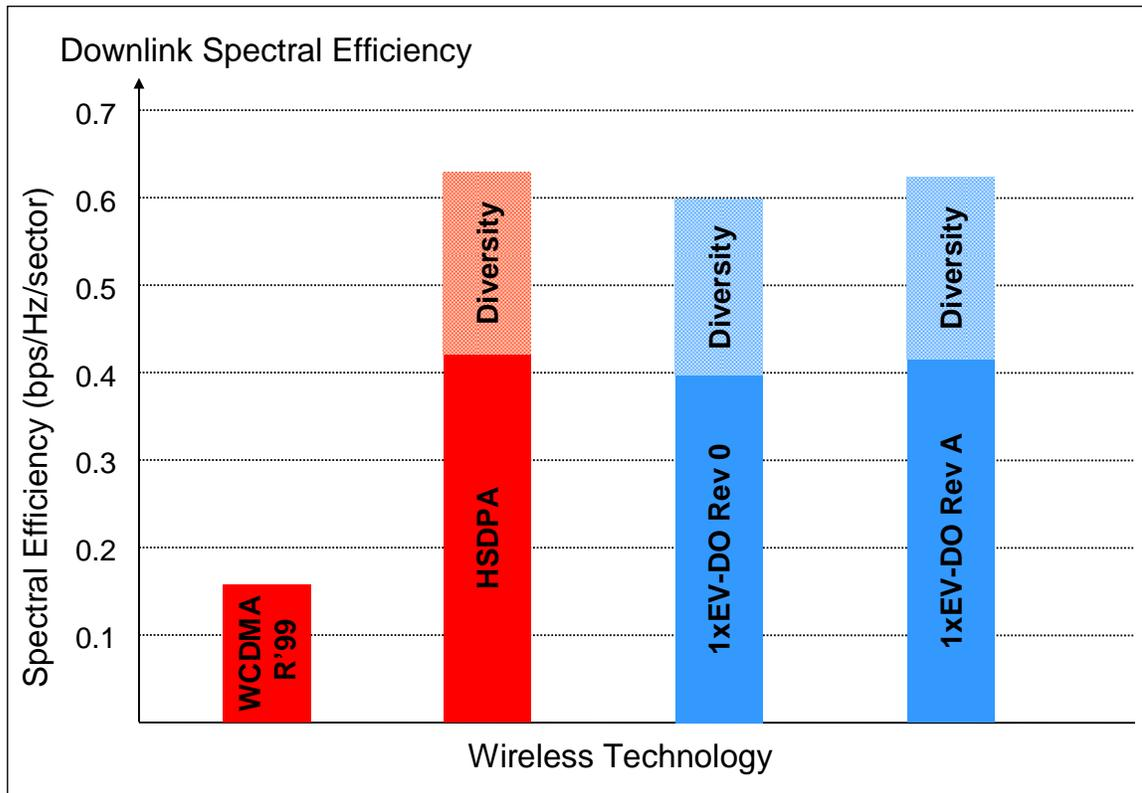
Mobile receive diversity provides a spectral efficiency gain of 50% for all technologies. HSDPA provides a spectral efficiency gain of approximately 2.5 times that of WCDMA Release 99. HSDPA and 1xEV-DO have fairly similar spectral efficiency. Relative to HSDPA, IEEE 802.16e, as shown in Figure 17, achieves similar or slightly higher spectral efficiency depending on the number of optimizations that are implemented, and assuming that no advanced antenna systems are used.
