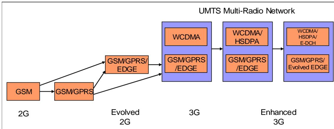
GSM operators first enhanced their networks to support data capability through the addition of GPRS infrastructure, with the ability to use existing cell sites, transceivers and interconnection facilities. Operators who deployed GSM more recently installed GSM and GPRS simultaneously; these include AT&T Wireless (now part of Cingular), Cingular Wireless, Rogers Wireless, and Telecom Personal.
