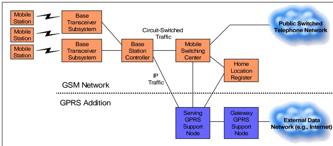
GPRS is essentially the addition of a packet-data infrastructure to GSM. The functions of the data elements are as follows:
