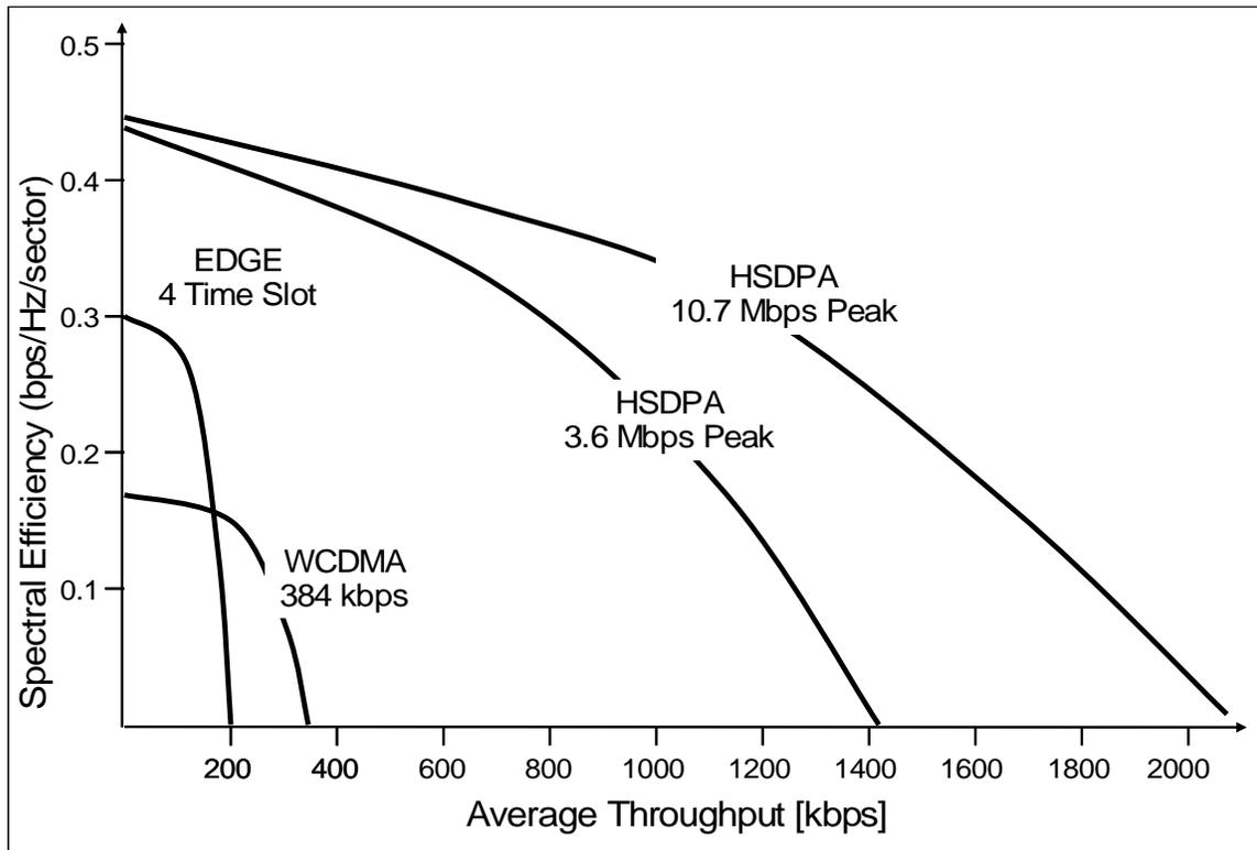
Note that spectral efficiency decreases with increasing average throughput, due to scheduling inefficiencies. This is the case for most wireless technologies. For average throughput, the simulations show that EDGE has high spectral efficiency for data rates below 100 kbps. For data rates above 100 kbps, WCDMA has greater spectral efficiency. But in all instances, HSDPA has the highest spectral efficiency.
