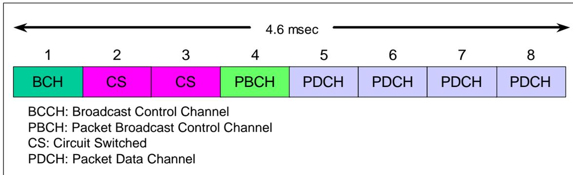
**Figure 3: Example of GSM/GPRS Time Slot Structure**
