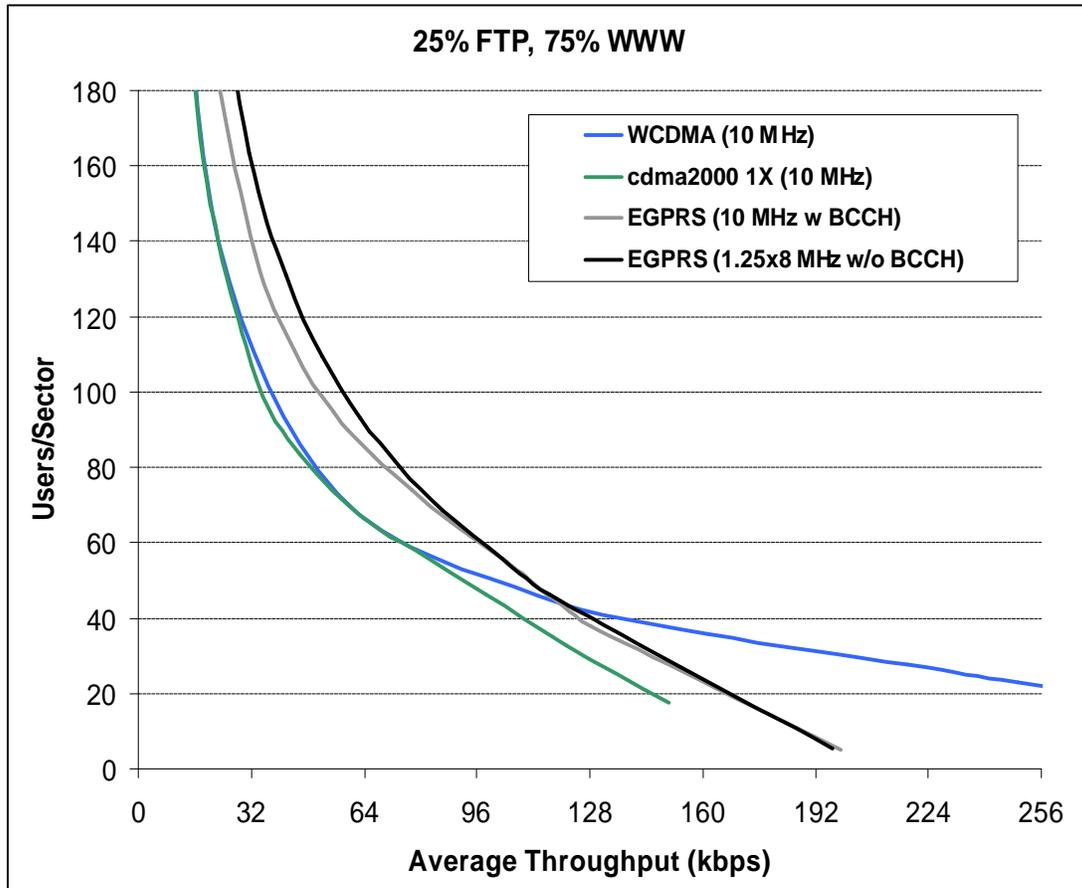
**Figure 10: Users per Sector in 10 MHz versus Average Throughput<sup>23</sup>**
