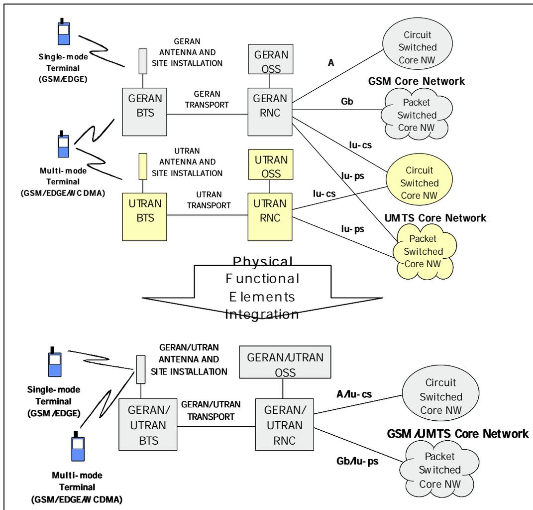
**Figure 12: Integration of UMTS and GSM/EDGE Core Network Equipment<sup>25</sup>**
