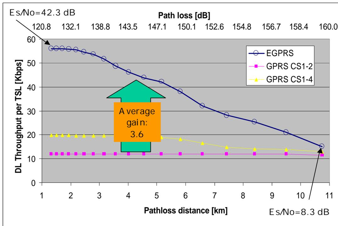
**Figure 4: Throughput Versus Distance for EGPRS/EDGE<sup>11</sup>**
