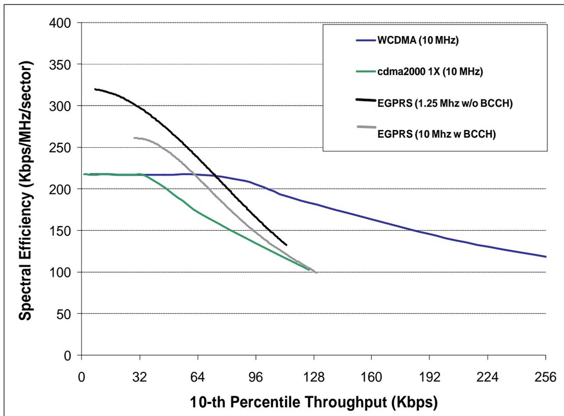
**Figure 9: Spectral Efficiency Comparison Based on 10-th Percentile Throughput<sup>22</sup>**
