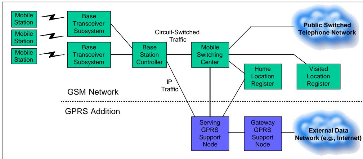
**Figure 2: GSM/GPRS Architecture**
