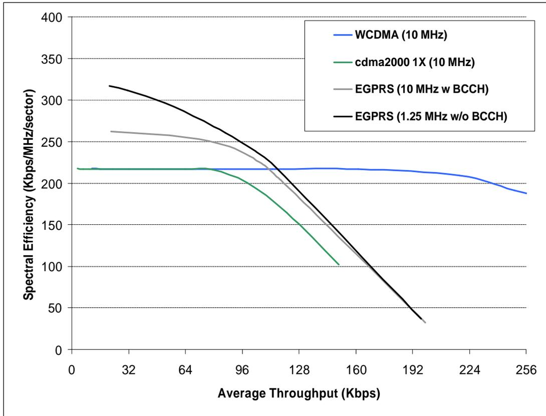
**Figure 8: Spectral Efficiency Comparison Based on Average Throughput<sup>21</sup>**
