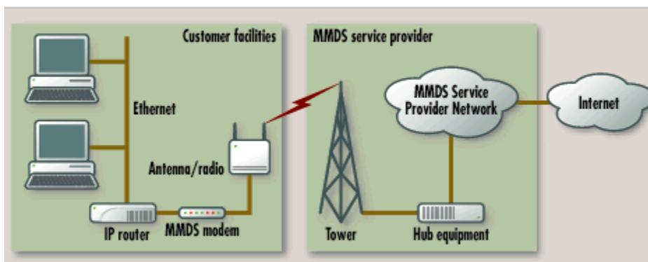
The ISP's tower is a hub in a point-to-multipoint architecture that multiplexes communications from multiple users. This approach differs from many other broadband wireless connections that operate on a point-to-point basis. The tower has a backhaul connection to the carrier's network, and the carrier network interconnects with the Internet. This architecture is fundamentally the same as other ISP connections, with the wireless link directly replacing a DSL, dedicated T1 or frame-relay link.
