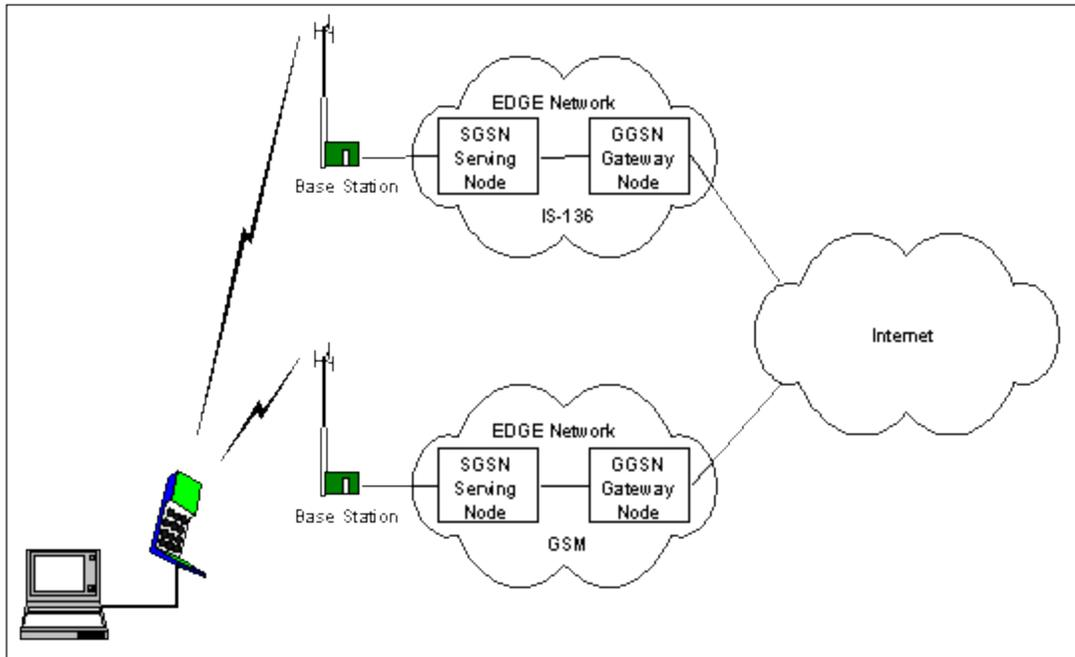
**Figure 2: The same EDGE wireless device will be able to communicate across both IS-136 and GSM networks.**
