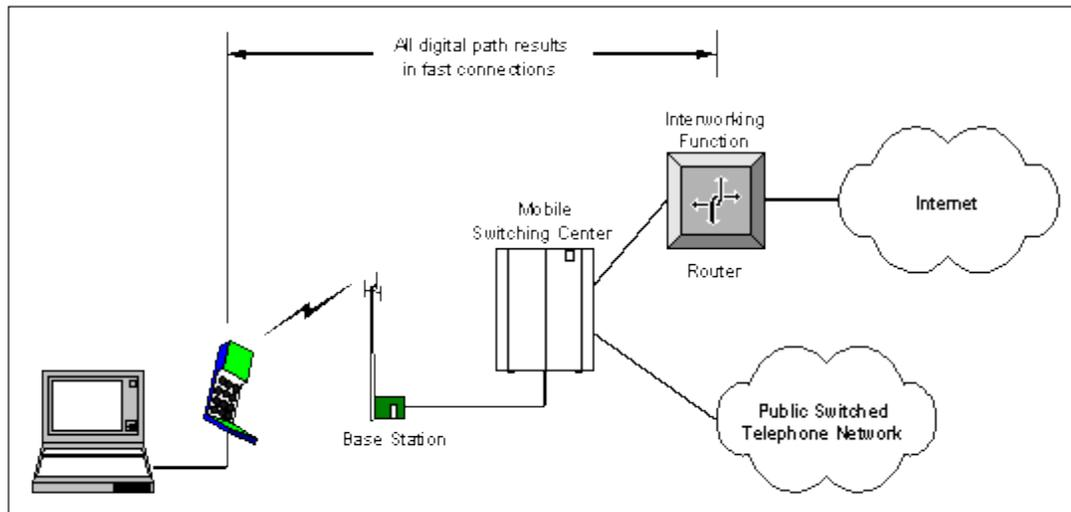
**Figure 3: QuickNet Connect for CDMA**
