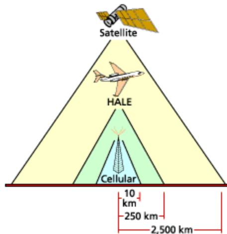
Figure: High altitude long endurance system with airplane as base station.
