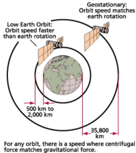
Figure: Geosynchronous versus low earth orbit satellites.
